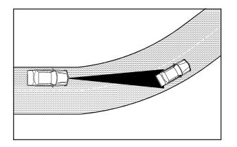
Adaptive Cruise Control may detect a vehicle that is not in your lane and apply the brakes.
